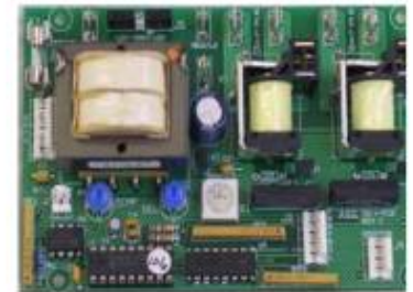
DS-4 Automatic Local Controller which is integrated into the Power Distribution Panel
