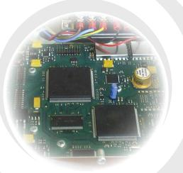
UHP-1100 is implemented as a compact single card ideal for integration into third-party OEM products. It is fully compatible with any other satellite routers of the UHP series. The router card has LED indicators, SMA or F type IF connectors and user LAN interface. Optionally, the router card can be equipped with the asynchronous LVTTL data port. Low power consumption and uniquely fast start upon power-up facilitate use of alternative power sources, such as solar batteries.
