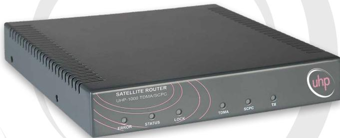
UHP-1000 router is a compact and reliable device and can be installed on a work desk or in an equipment rack or inside a customized enclosure. Low power consumption and uniquely fast start on power-up facilitate use of alternative power sources, such as solar batteries. Integrated high-performance IP router supports different protocols and has expanded means for provision of Quality of Service (QoS).
