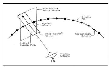
satellite has been stored in the RC2500, finding it again is as easy as locating a fixed satellite. Simply move to Auto mode, select the satellite from the list of those available, specify the proper polarization and let the RC2500 do the rest.
