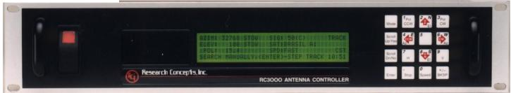
Avoid the time consuming tasks of manually positioning your mobile antenna and tracking inclined orbit satellites. The RC3000 allows even non-technical personnel to automatically locate and position a mobile antenna within minutes from power up.
