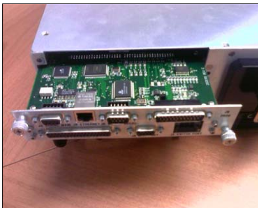
Removable rear panel monitor and control card
