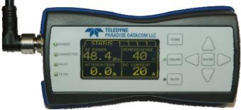
This device allows the operator to adjust the attenuation of the connected unit, and control the mute/unmute selection, as well as monitor the status, conditions and settings of the connected unit via a serial RS-485 connection. Fault conditions and other events are tracked in the controller's internal log.
