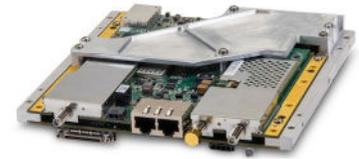
ST Engineering iDirect's 9-Series modems provide a superior level of IP broadband capability, supporting DVB-S2/ACM and Adaptive TDMA and are designed for high-bandwidth fixed and mobility applications. The 9-Series has enhanced performance, efficiency and security with FIPS 140-2 Level 3 certification and supports both one-way and two-way TRANSEC to enable mission-critical communications.
