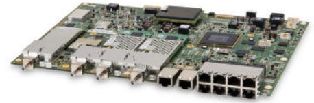
ST Engineering iDirect's 9-Series modems provide a superior level of IP broadband capability, supporting DVB-S2/ACM and Adaptive TDMA and are designed for high-bandwidth fixed and mobility applications. The 9-Series has enhanced performance, efficiency and security with FIPS 140-2 Level 3 certification and supports both one-way and two-way TRANSEC to enable mission-critical communications.
