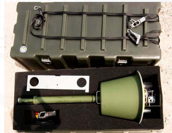
Photo representing a dual optic feed system
