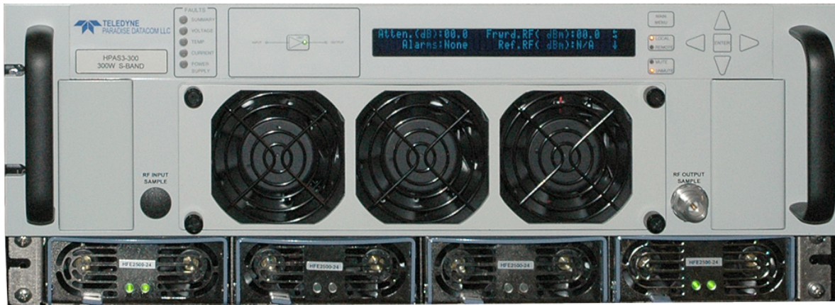
300W S-Band 3RU SSPA Chassis with 1RU N+1 Power Supply
