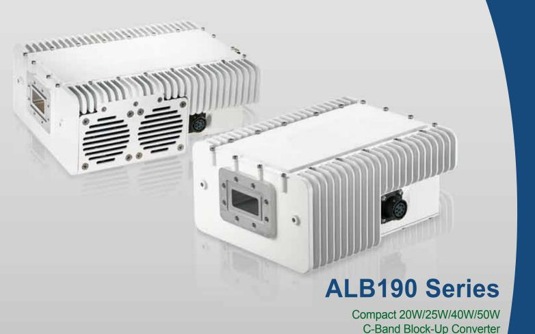
This small and lightweight BUC is ideal for mobile and satellite uplink applications. Designed to be mounted on the feed horn, the BUC has excellent efficiency and consumes less than 250W for 50W C-Band BUC. The unit works on a wide range DC power supply of 38V to 60V. The BUC is able to work up to 60°C. Innovative and efficient thermal design makes this BUC one of the smallest, lightest and most reliable in the industry.
